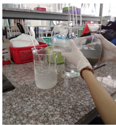
▲ Fig.5. Washing fly ash
